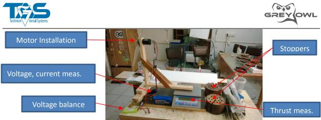
Figure 11- Static thrust testing
