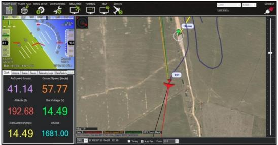
Figure 26 - Flight Data tab of the APM Mission Planner
