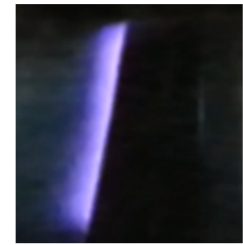
Figure 1: Left figure: Schematic illustration of an SDBD plasma actuator. Right figure: Ionized air over an electrode covered by dielectric layer, at atmospheric pressure. The electrodes are made of aluminum tape, and the dielectric layer is a 1 mm perspex sheet. Photo taken at the Wind Tunnel Labs of the Technion's Faculty of Aerospace Engineering.
