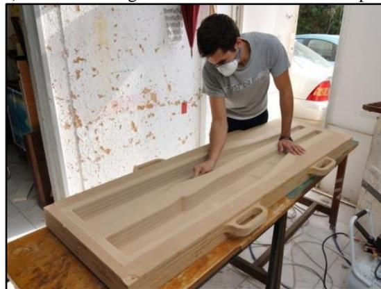
Figure 8 - Fuselage Lay- Up and manufacturing Tool
