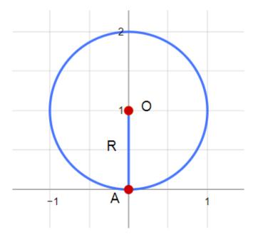
During the rolling of the circle, point A moves around the center O. Define  $\theta$  as the angle between the segment OA, and the initial segment when A(0,0). The length of OA is R as it is the radius of the circle. The center O position changes with respect to  $\theta$  as the circle performs a pure roll by the following equations:
