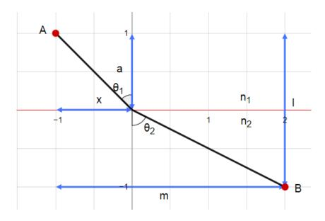
The velocity in the mediums  $n_1$ , and  $n_2$ , are  $v_1$ , and  $v_2$  accordingly.
