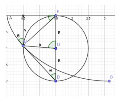
Since the cycloid is created from a rolling circle with a radius R, at any given time F is the instant center of rotation of the circle, so every point on the circle rotates around F at that moment and performs a circular motion around that point. M moves in a circular motion with respect to F at any given time, so it's velocity is perpendicular to the line MF. The
