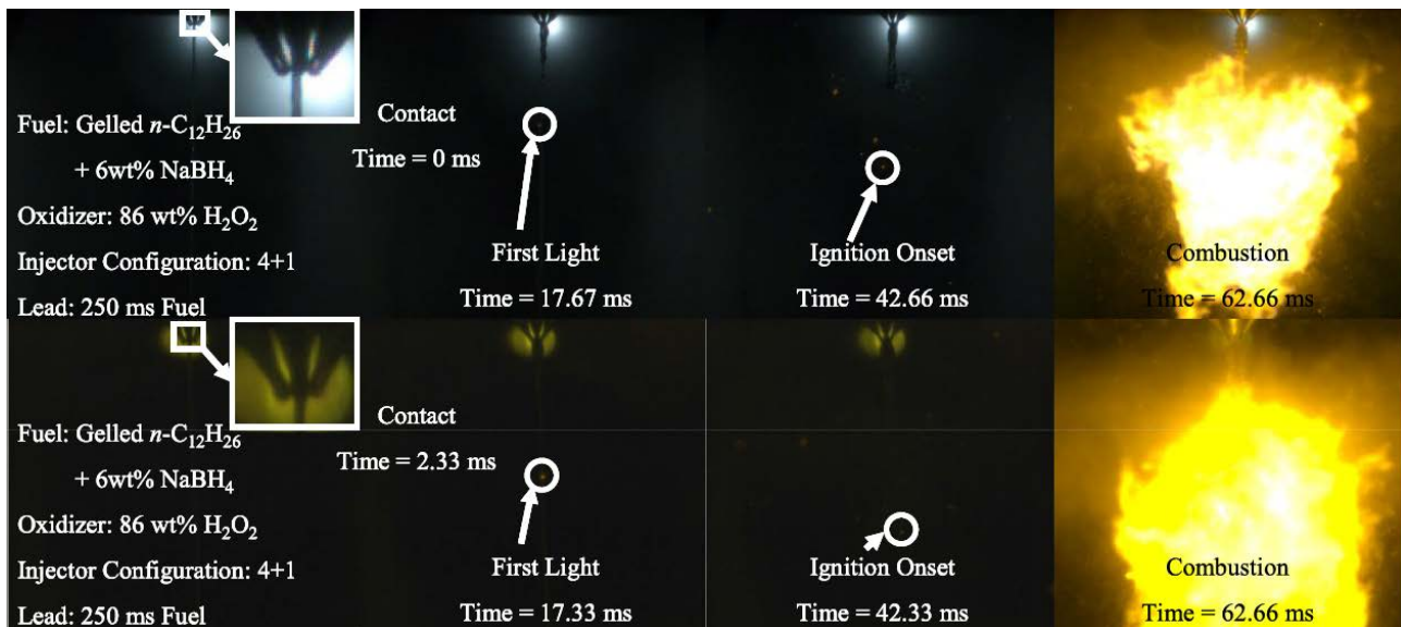
Figure 5 – Images of "First Light", "Ignition Onset" and combustion of hypergolic gelled fuel with HP.
