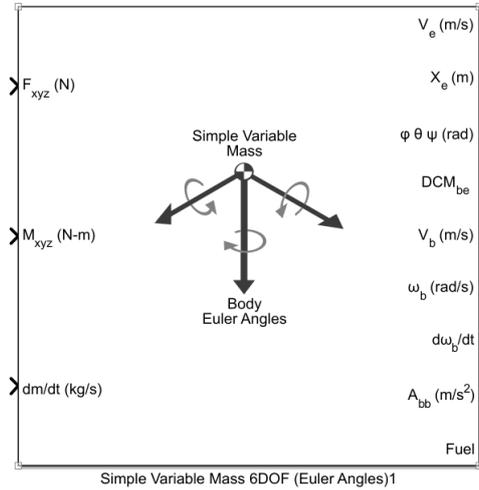
Figure 3: simple variable mass 6DOF Euler Angles block
