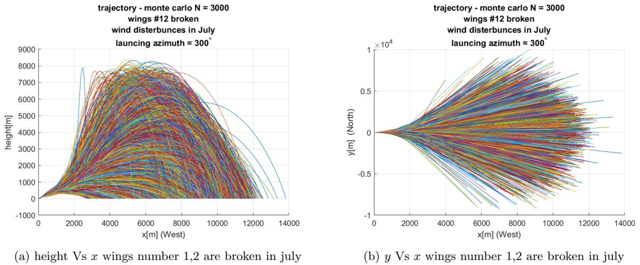
Figure 20: *Monte Carlo* trajectories for wings number 1,2 are broken in July
