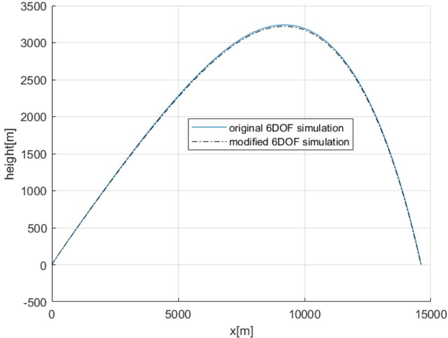
Figure 12: trajectory of the modified 6DOF Vs the original 6DOF
