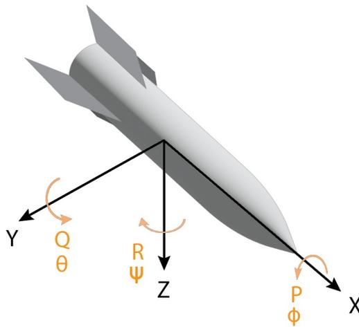
Figure 1: body axes
