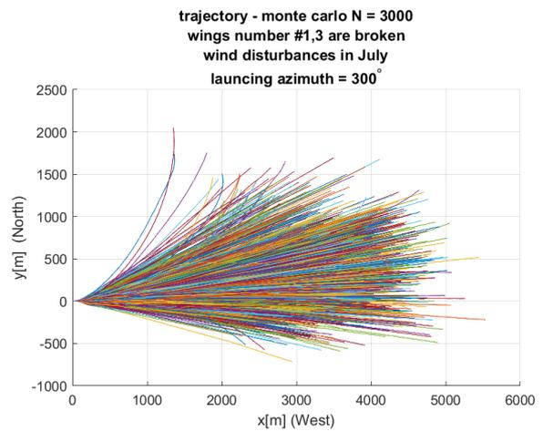
(b)  $y$  Vs  $x$  wings number 1,3 are broken in July
