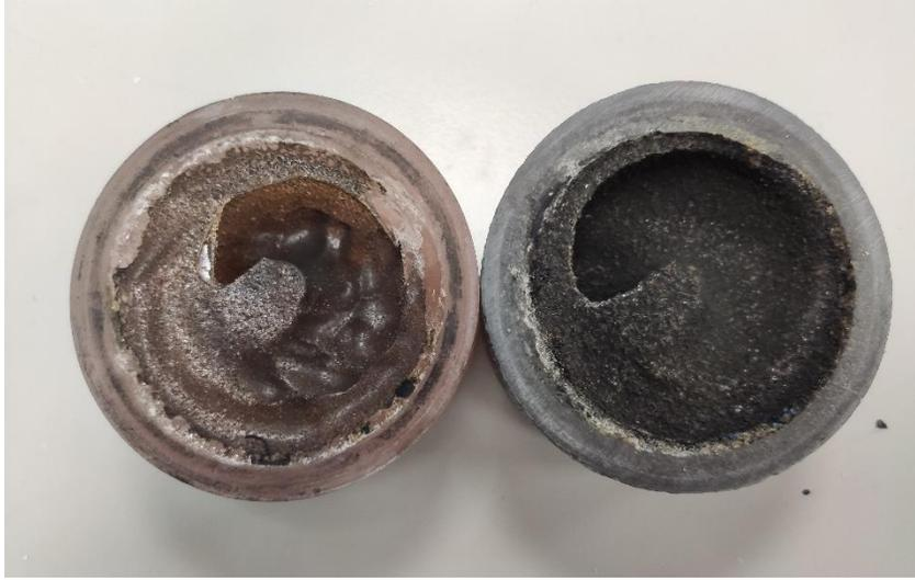
Fig. 14 Post burn photos of plain polyester (left) and polyester and 5% EG (right) with helical port.
