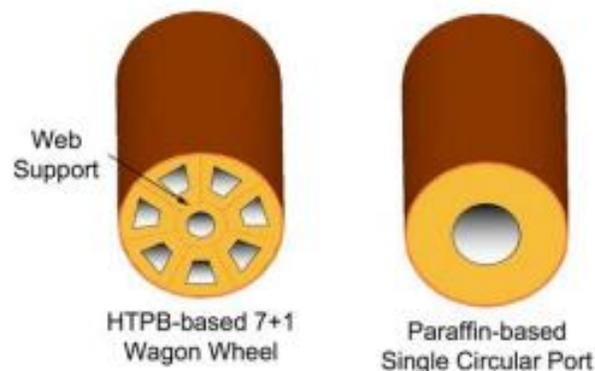
Fig. 3 Multiple port and single port designs [6]
