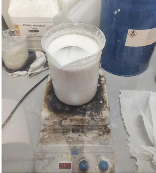
Fig. 11 Dissolving the casting mold
