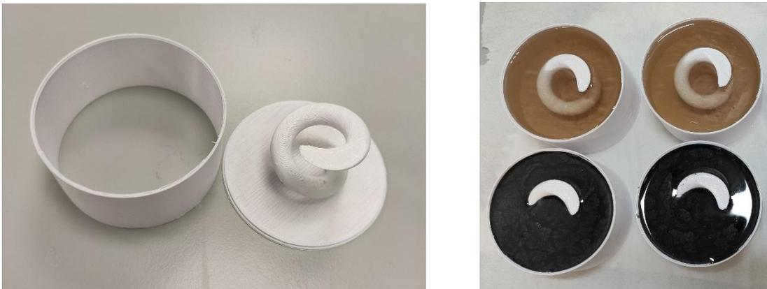
Fig. 10 (left) Helical fuel port casting mold; (right) Casted fuel mix, upper row plain polyester, bottom row polyester with 5% EG.
