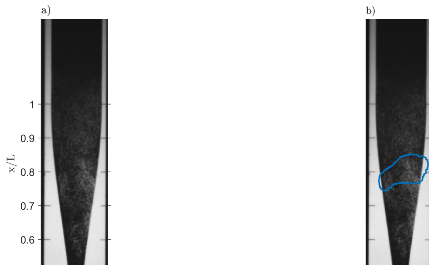
Fig 5 -Example of shockwave perimeter detection. a) raw image of diverging part of CD nozzle for JP-5 at p_b/p_0 = 0.25 . b) higlighted perimeters of the detect bubbly-shocks.
