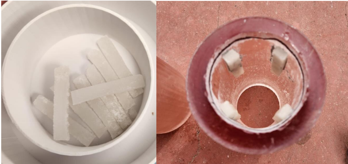
Figure 17- On the left image we see casted solid propellant, after being separated from its mold, the rough texture can be explained by insufficient mixing, showing some areas with high content of AP grains. On the right we see a casted fuel grain, after being separated from its mold and with solid propellant glued on.
