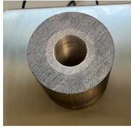
Fig. 6: 2 nd Sub-Experiment Fuel Grain (inner layer plain polyester, outer layer polyester with 5% EG)
