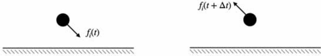
Figure 4: Illustration of the bounce-back boundary condition of a fluid particle on an arbitrary solid wall.
