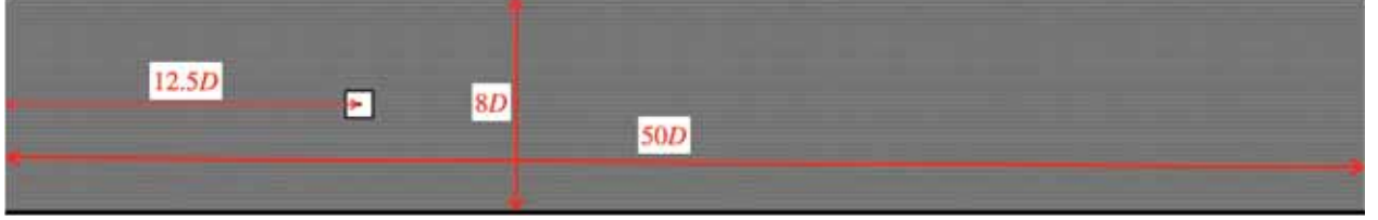
Figure 12: Computational domain of the two-dimensional square in a channel.
