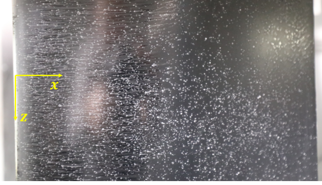
Figure 6: Example of streamlines from oil visualization obtained at freestream U = 40 m/s.
