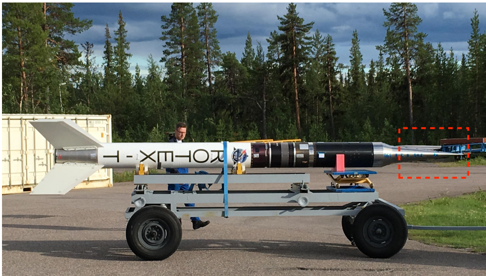
Figure 1: ROTEX-T hypersonic vehicle model during roll-out (DLR, 2016) - conic forebody highlighted in red.
